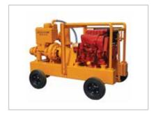
Oasis OP Model provides a wide selection of low & high output pumping systems designed for on-site dewatering applications. The pumps provide continuous high discharge flow and discharge head. OP models use closed type single stage heavy duty impellers and are self-priming, vacuum assisted pumps made for strenuous duty.
